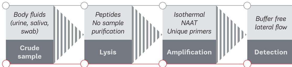
The technological invention of Selfdiagnostics is a combination of a robust sample preparation, specific DNA detection and isothermal amplification with a simple lateral flow visualisation combined with self-regulating micro-heater and operated by passive microfluidics. Each invention possesses an innovative approach to contribute to the entire platform. Sample preparation with carefully selected lysis agents allow direct amplification within the sample, avoiding complicated sample purification
